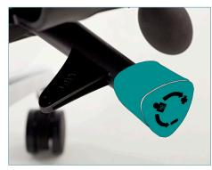
Turn hand wheel clockwise to increase tension to compensate for body weight, anti-clockwise to decrease. This hand wheel is found on the right hand side underneath the seat next to the seat height adjustment lever.
