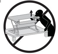
Warning: Impact Hazard! Worksurface under tension. Moving Parts can Crush and Cut. Raise worksurface to top of vertical adjustment BEFORE removing equipment. Failure to heed this warning may result in serious personal injury and or property damage!
