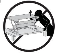
Warning: Impact Hazard! Moving Parts can Crush and Cut. Raise worksurface to top of vertical adjustment BEFORE removing equipment. Failure to heed this warning may result in serious personal injury and or property damage!
