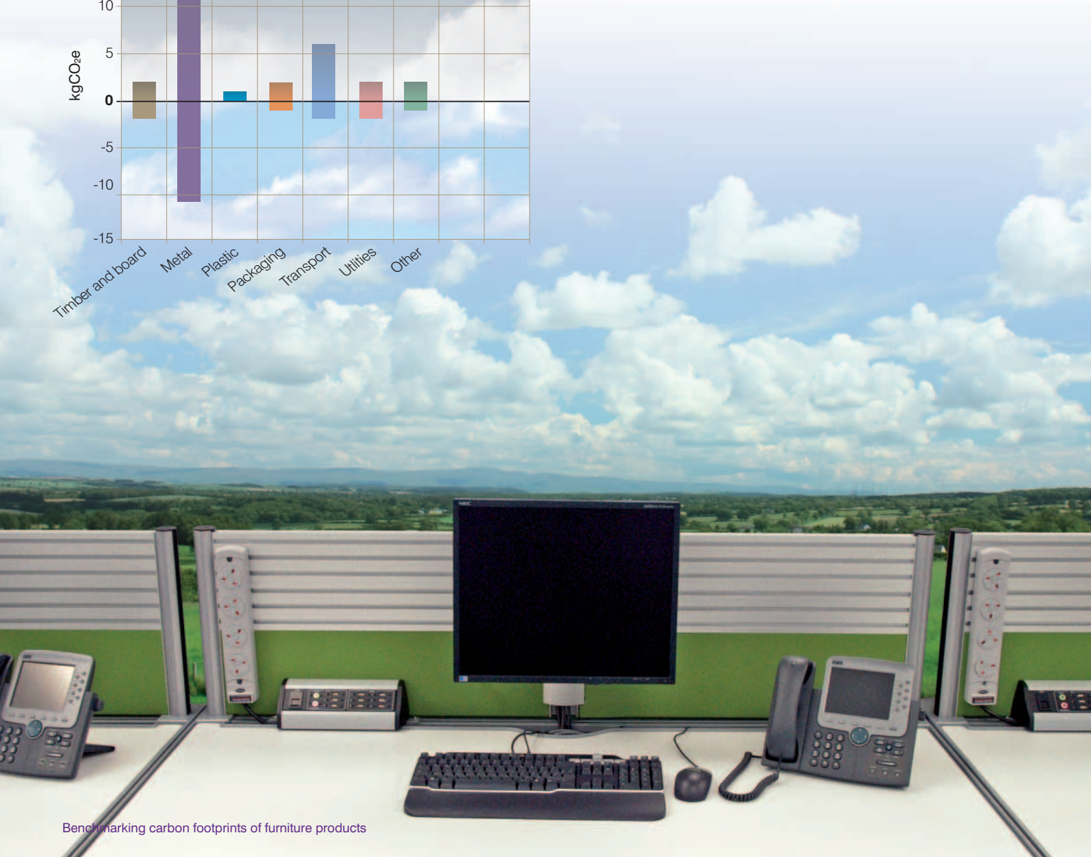
Figure 12 Data variation for each category of carbon footprint input to the average carbon footprint for the rectangular desk. The zero value on the graph represents the average carbon footprint.
